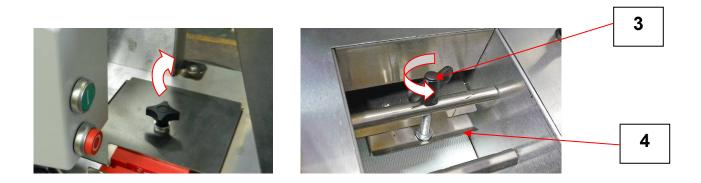
4 Remove cover on top behind hopper. Loosen wing bolt (3) and lift out rear scraper (4). Wipe clean and refit.
