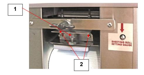
3 Turn down knurled bolt (1) and withdraw front scraper from retaining hooks (2). Wipe clean and replace.
