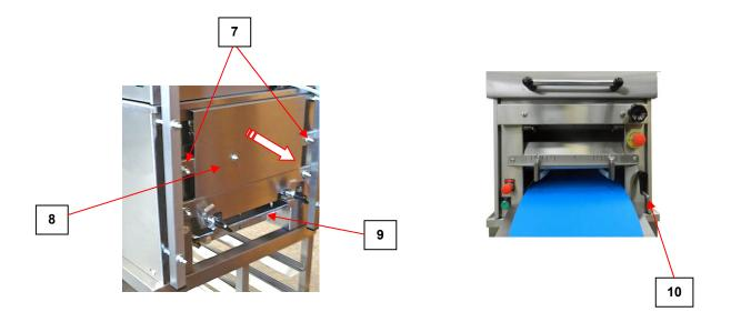
12 Remove pressure board (9) by winding handle (10) to move the board to its lowest position. Lift it out of its slots and slide the board out from the front of machine. Wash board in solution of sterilising solution and hot water. Dry thoroughly.
