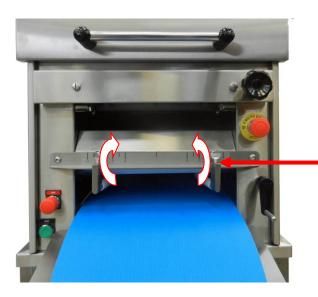
CHECK THE DIRECTION OF THE MOULDING BELT TRAVEL BEFORE COMMENCING PRODUCTION
