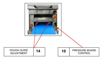
The pressure board dough guides (14) are adjusted by means of the guide clamps. The length of the dough piece required determines the width at which the dough guides are set. It should be noted that the dough guides and pressure board adjustments are relative to each other and should be adjusted accordingly.
