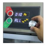
**Control panel**Allows the user to choose the thickness and number of slices
