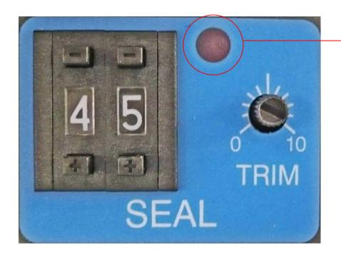
Pulse light. This comes on when the sealing wire is powered
