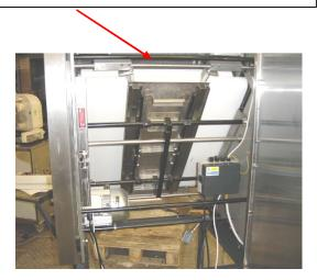
4. Clean and replace chain by dropping down conveyor from the back and clipping in place at the front. (Reverse of removal).
