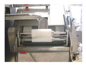
**3.** Pull out and down, large hopper area sheeting to expose rollers.
