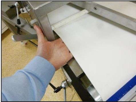
Upper Belt Tensioning
