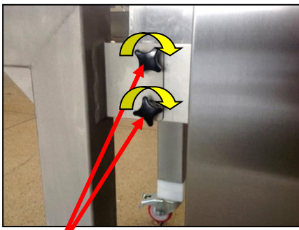
Use the Two Black Thumb Screws to Secure the Connecting Plates on Both Sides of the Machines
