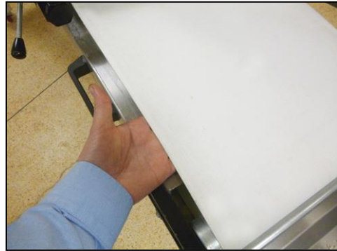
Lower Belt Tensioning
